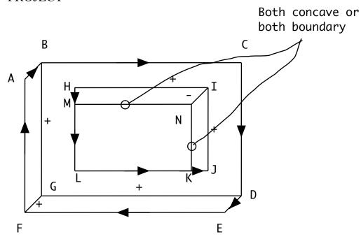
We can go no further. The Waltz procedure has uncovered a genuine a genuine ambiguity - is the center area (bounded by K,L,M,N) a solid bottom or a hole? Further data would be needed to settle this. (E.g. if this area were a different color or shading from the background, it's probably a bottom; if the same as the background, probably a hole.
