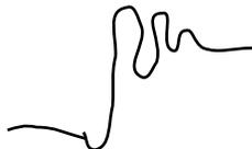
This behavior (known as “ringing”) is a consequence of the physical transitions occurring inside the transistors from which the gate is constructed.
